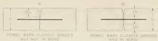
FIGURE 41.—PLANE-OF-WEAKNESS JOINTS DESIGNED TO PERMIT FREE WARPING.
